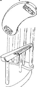
TH29 pictured with locks attached to the underside of the tray and tracks attached to the outside of each chair arm. **NOTE:** Locks and tracks are "rights" and "lefts"; A total of four hardware pieces are required for this mechanism to function safely. TH29 is packaged as a full set of tracks, locks and attaching fasteners.
